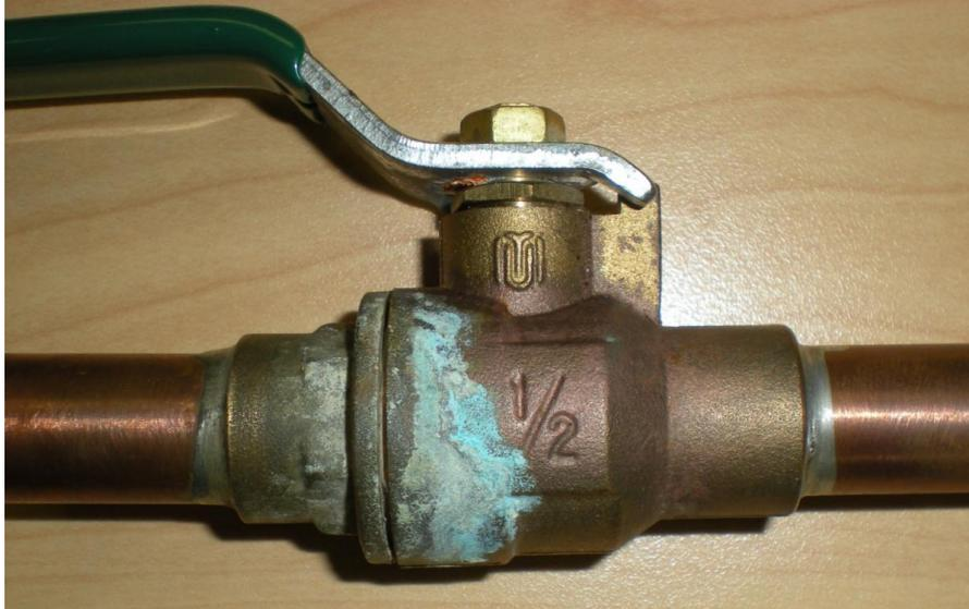
Brass products are more susceptible to damage from dezincification under certain water conditions. Bronze valve alloys are more rugged, and have been proven to be less likely to have any corrosion issues. Either brass or bronze will render excellent service when utilized properly. Both materials are available from Milwaukee Valve for their extensive lines of gate, globe, check and ball valves. Every one of these valves has been designed with the specific materials of construction in mind.
