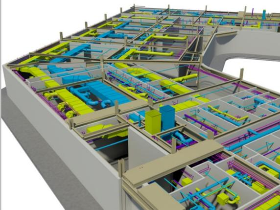
The BIM toolset helps automate clash detection of elements, such as piping or electrical conduit or ductwork that runs into a beam. By modeling all of these things first, clashes are discovered early, and
