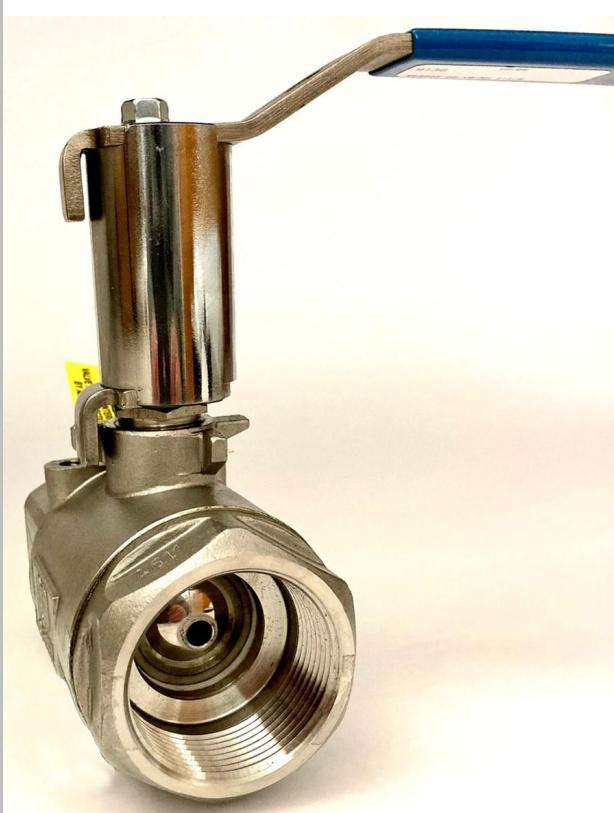
The most widely held understanding of a “vented ball” is one in which a relief hole is drilled in the upstream side of the ball (the Milwaukee Valve –VB option). When the valve is closed, any media inside the valve has a path to “vent” to the upstream piping. Many industrial applications have temperature fluctuations that can cause significant increases in cavity pressure, potentially
