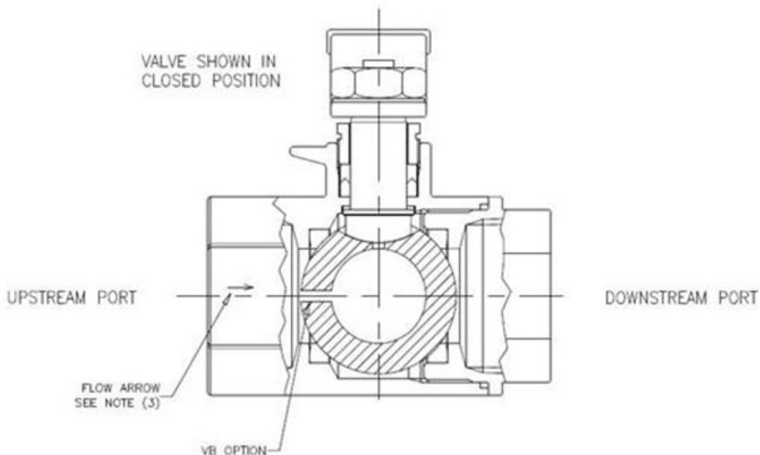
Commonly, the error is made when referring to the hole in the stem slot of the ball as a “vented ball”. To be sure, this hole will allow any increase in internal cavity pressure to equalize to the adjacent piping, but only when the valve is open. When the valve is closed, the media can get from the body cavity to the inside of the ball, but not past the pressure seal of the seats.
