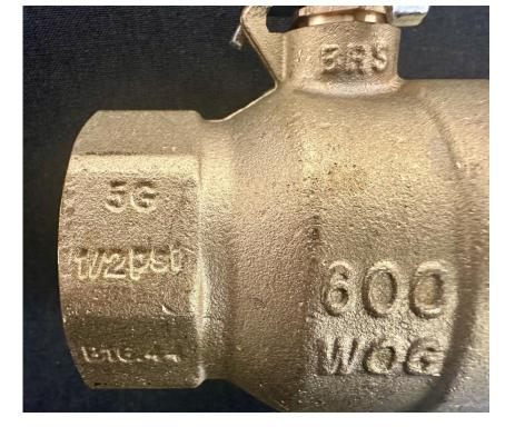
B16.44 does not apply to manually-operated gas valves which are an integral part of a gas appliance. These integral gas valves are subject to the American National Standard for Manually Operated Gas Valves for Appliances, Appliance Connector Valves, and Hose End Valves, ANSI Z21.15/CGA 9.1 ANSI Z21.15 states that "A permanent marking specifying the maximum pressure rating of 1/2 **PSIG** (3.5 KPa) shall be provided on each valve".
