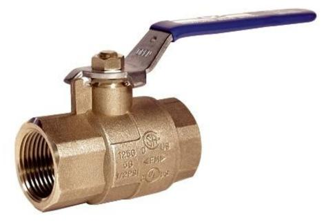
The 5G mark signifies that the valve meets the requirements of <u>ASME B16.44</u>. B16.44 applies to quarter-turn, manually-operated metallic valves, intended for indoor installations as shutoff valves when installed in above-ground, fuel gas piping, downstream of the gas meter outlet and upstream of the inlet connection to a gas appliance. The valves covered by B16.44 are limited to application temperatures between 32° F and 125° F at pressures not to exceed **5 PSIG**.
