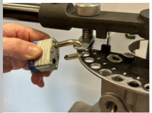
A lock link can be fieldinstalled to provide locking of the valve in any of the 10 positions of the latch plate. If required for a project, this option can be installed prior to shipment.
