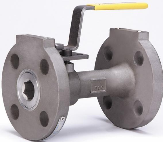
For this example, let's use the F90/91 series of flanged ball valves. Under the available body materials is a listing for ASTM A351/A744 GR CF8M. The A351 and A744 are material standards for castings that the valve bodies meet.
