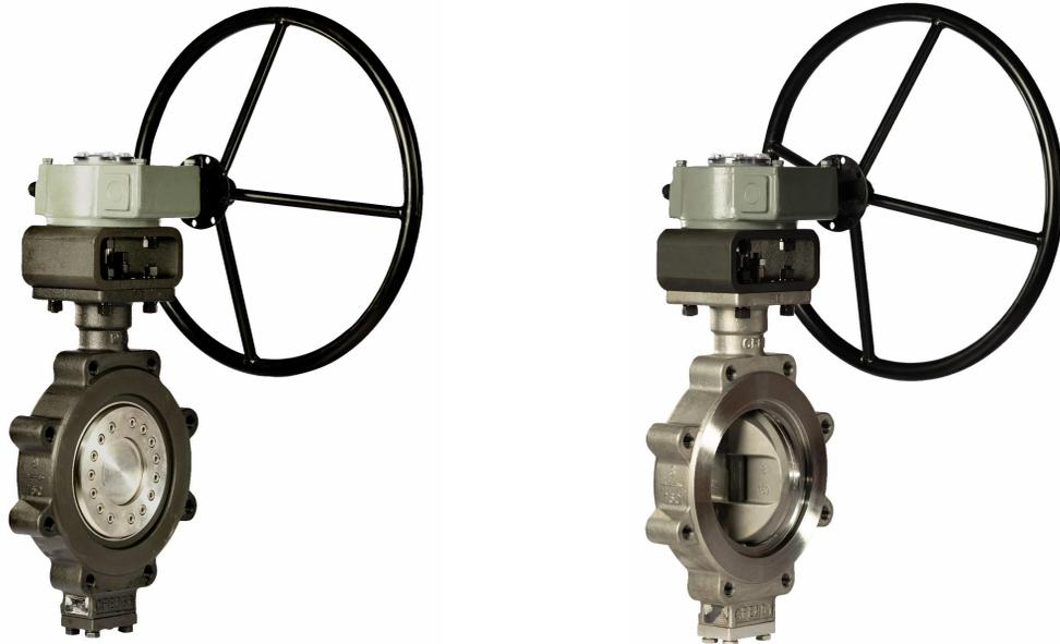
Triple offsets are generally used in applications where gate valves are found, where a metal seat is required, and tight shutoff and/or quarter-turn actuation is desired. Applications such as high-pressure steam (over 150 PSI), superheated-steam, high-temperature gases and oils, and other high-temperature applications are good for this type of valve. The triple offset valve is used in many similar industries as the double offset butterfly valve, but the applications are more demanding.
