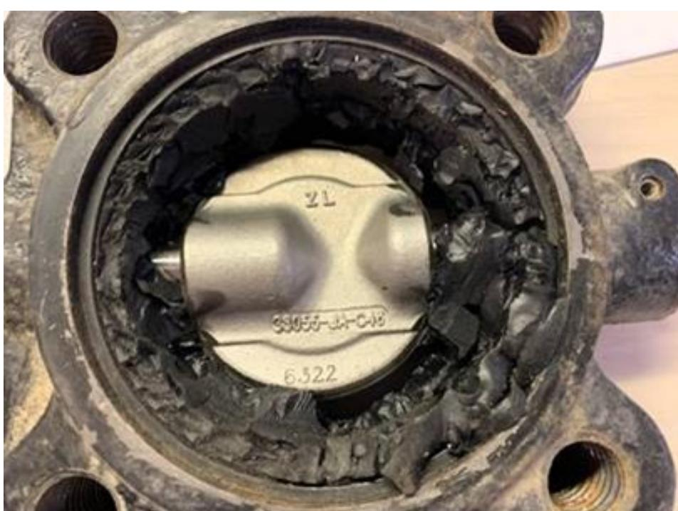
3. This valve was reportedly used on Jet A Fuel / Purge Oil. These are different media, so we're not sure which one did the damage. Regardless, EPDM would not be
