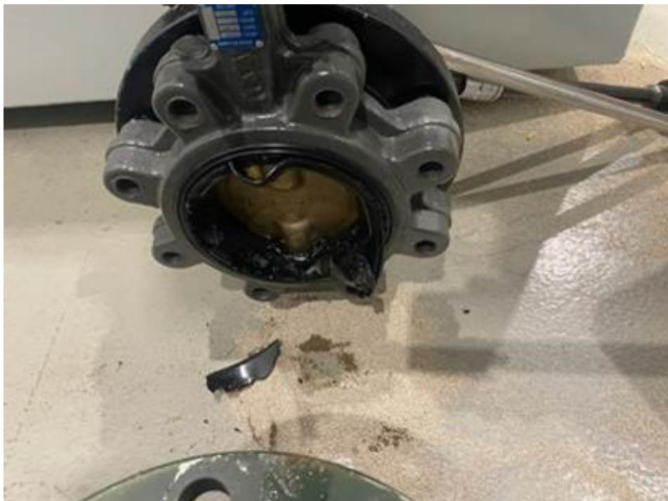
2. This valve was installed on a Purge Oil line. Purge Oil is used to preserve fuel tanks of jet aircraft when not in use for extended periods of time. Purge Oil is described as Petroleum Distillates, Hydrotreated Light, per the Material Safety Data Sheet (MSDS) that was supplied with the returned valve.
