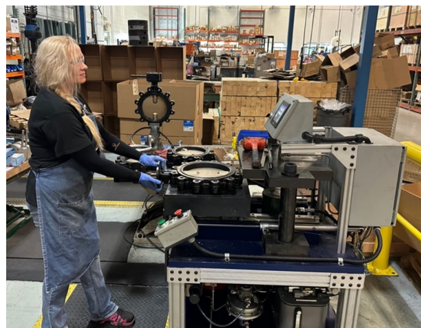
Milwaukee Valve's Michelle Scukanec prepares an M-Series butterfly valve for Shell and Seat testing in the New Berlin assembly and warehouse facility.
