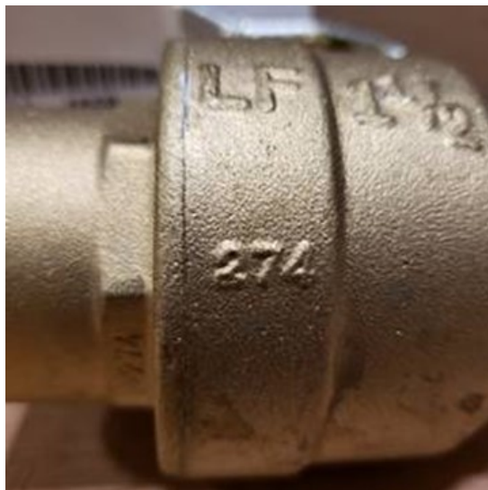
1½" UPBA-485B Markings – "274" ASTM B583 C27450 (Body and Tailpiece)
