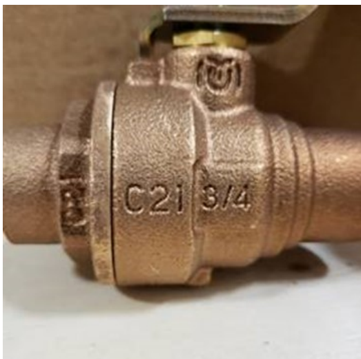
3/4" UPBA-150 Markings – "C21" ASTM B584 C89833 (Body and Tailpiece)
