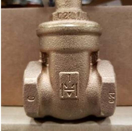
1" UP148 Markings - "C21" ASTM B584 C89833 (Body and Bonnet)
