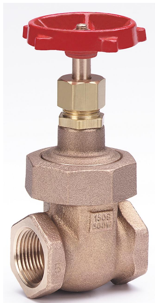
The 1141 gate is a union-bonnet gate. This valve CAN BE repaired in the field.
