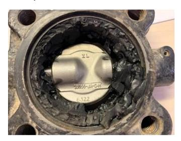
2. Butterfly valve with EPDM liner installed in ULSD (Ultra Low Sulfur Diesel) Fuel line.
