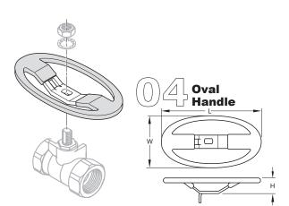
Oval handles can also prevent accidental valve operations, since they have less projection than a lever handle, and require more turning force to operate. OSHA requires the use of oval handles in many installations for safety reasons.
