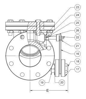
Note 1: On pump discharge, the preferred check valve is either an in-line spring loaded valve or a swing design with lever and weight. Install these valves as far as possible from the pump and elbows with a minimum distance of 5 times the pipe diameter.
