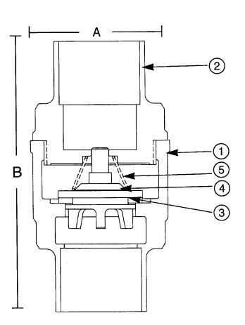
**Note:** Check Valves may be installed in both the horizontal and vertical lines with upward flow or in any intermediate position.
