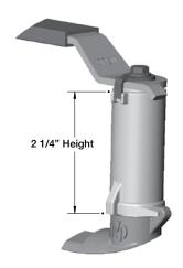
Oval handles can be installed where a standard lever handle might encounter interference from adjoining piping. Oval handles can also prevent accidental valve operations, since they have less projection than a lever handle, and require more turning force to operate.
