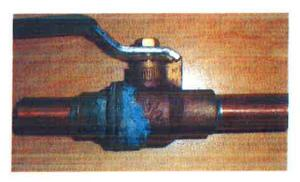
15%, there is risk for dezincification, and when it is below 15%, you are safe. Actually, dezincification can occur in *any* zinc-bearing copper alloy, depending on the circumstances, and when it happens it can be destructive even when the starting concentration of zinc is fairly low.
