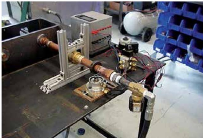
UltraPress® valves undergo a reverse bending/fatigue test, with superimposed alternating pressure spikes, to 250,000 cycles of bending with 250,000 [0-80-0] psig pressure cycles.
